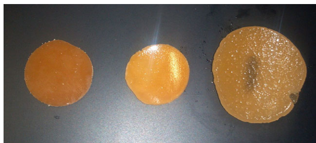
Figure 1. Illustration of dry poly(glutaric acid-glycerol) microcrystalline cellulose composite film (left) and poly(glutaric acid-glycerol) microcrystalline cellulose composite films after absorbing water (middle) or DMSO (right). [Color figure can be viewed in the online issue, which is available at wileyonlinelibrary.com .]
